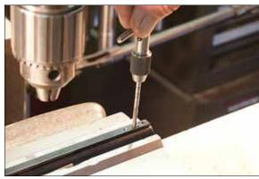
11. Finish hand-tapping with a 6-48 bottom tap. **Avoid tapping too deep & denting the barrel.**
