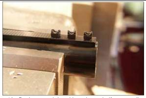
13. Back out each bead less than a half turn so all beads are all in alignment with the rib.
