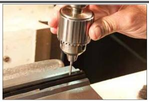
10. Lubricate & use a 6-48 starter tap to hand start all holes, use the mill to ensure the taps are vertical. **Avoid tapping too deep & denting the barrel.**
