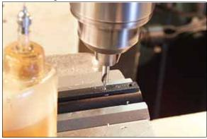
8. Drill starter holes at .375" intervals (center to center) forward of the first hole, one hole for each bead the customer wants installed.
