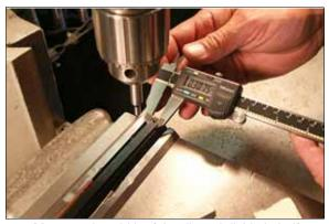
5. Measure the width of the rib and divide in half to locate the distance to center.
