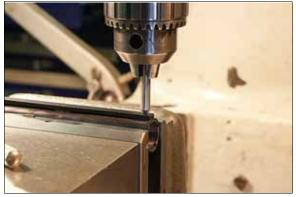
7. Locate the longitudinal starting point at the center of the existing bead hole. Zero the mill indicators.
