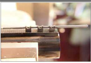
16. Again back off all beads less than a half turn from bottom and re-align all three beads with drill rod. Wait for the Lock-tite to set.
