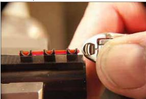
20. Briefly touch a lighter to the rear of the fiber-optic rod, forming the rear bulb and locking the rod in place between the front and rear beads.
