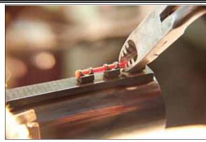
To quickly change sight color, cut the rod between the beads, remove the old rod, & repeat steps 17-21 to install a new rod color. Rod change takes about two minutes & requires only a cutter and lighter.
