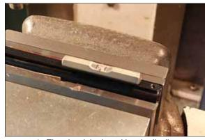
4. Then level the barrel longitudinally.
