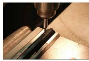
6. Locate the edge of the rib & move half the rib width (factor in the indicator width) to locate center.
