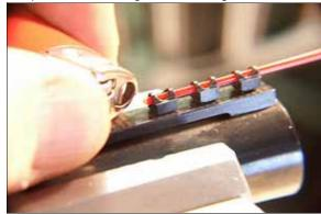
18. Briefly touch a lighter to the fiber-optic rod forming the front sight bulb.
