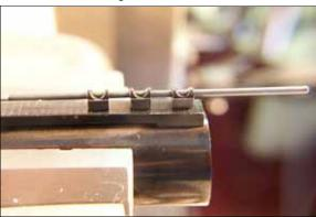
14. Use a length of 1/16th inch drill rod to confirm that all the beads line up correctly. If the bead holes are too tight, carefully run a 1/16th inch drill bit through the hole to de-burr an obstructions.
