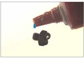
15. In turn, remove each bead, put a small drop of **blue** Lock-tite on the threads, and re-install the bead.
