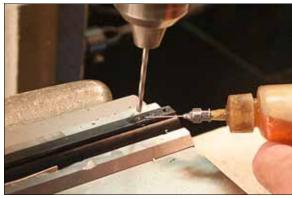
9. Lubricate & drill out all starter holes using a #31 bit. Re-drill the original hole if smaller than 6-48. **Do not drill too deep and drill into the barrel.**
