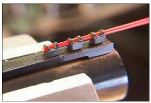
17. Insert the fiber-optic rod choice so that roughly 1/16th inch protrudes past the front bead. The longer the protrusion, the larger the resulting bulb.
